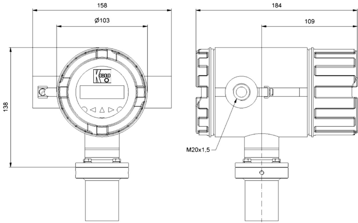
7.5.2 Sensor terminal box – remote mount transmitter
