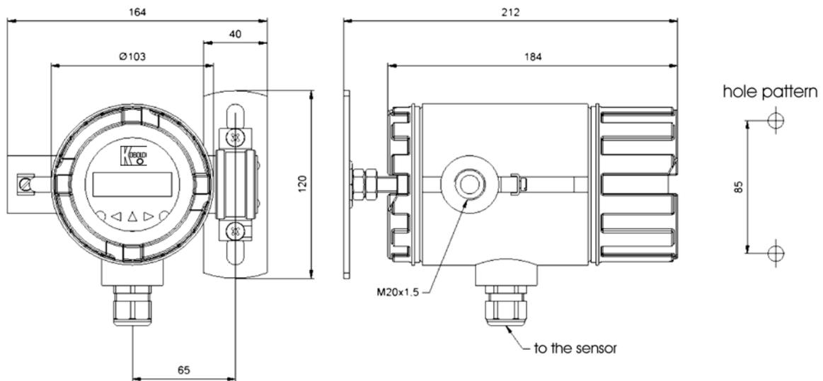
Transmitter type UMF2 with wall bracket
