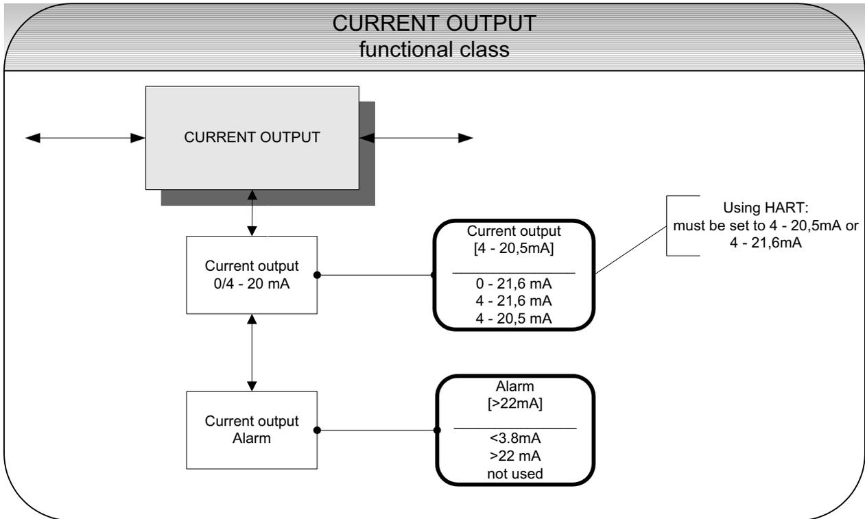
The current aoutput is always assigned to volume flow.
