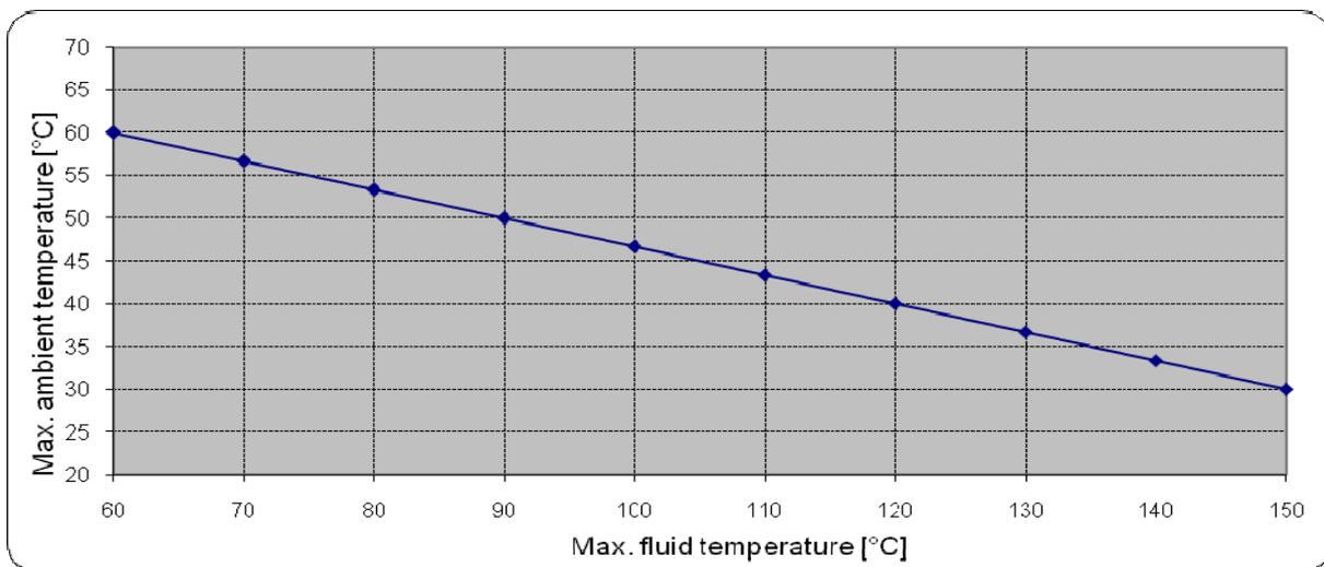
**6.6.1.2 Remote mount transmitter: sensor maximum ambient temperature depending on the fluid temperature**
