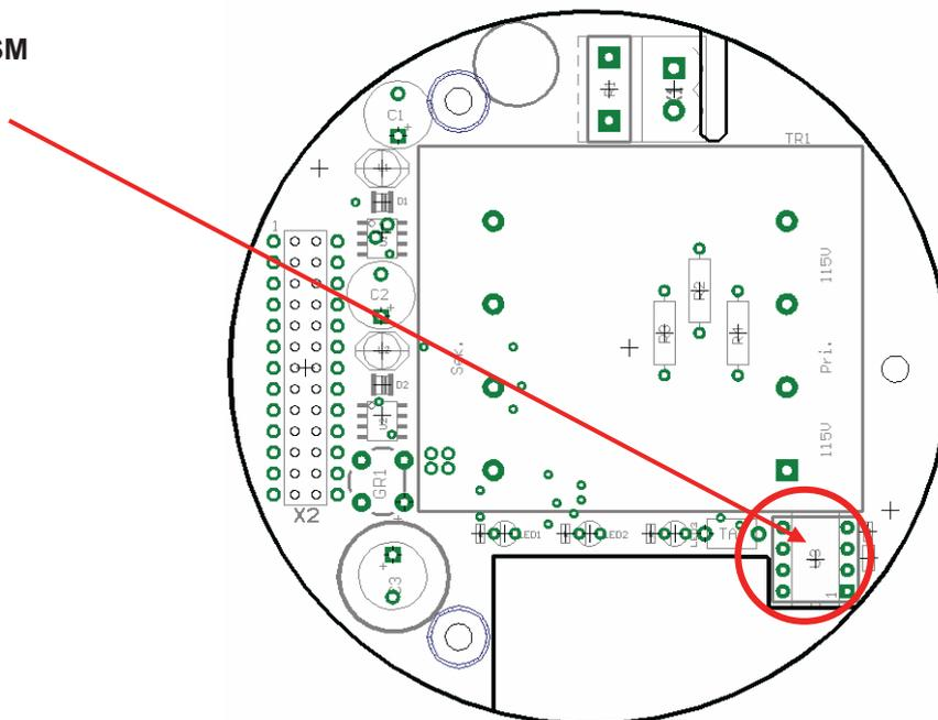
At any exchange watch the polarity of the memory chip. Pin 1 is signed by a dot or a notch.
