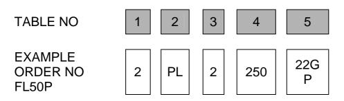
**Example Order No. =** Type FL50P ; double float ; Polypropylene plate process connection ; PVDF material ; 250mm long ; Glass Reinforced Polyamide connection head.
