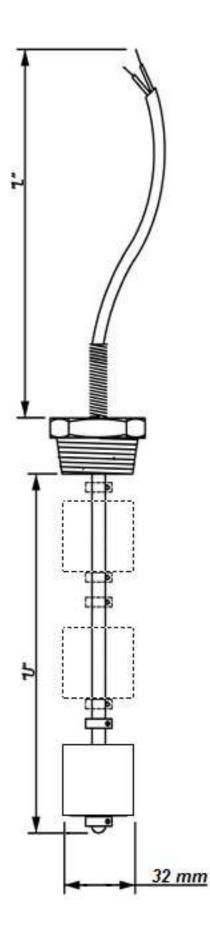
Type FL32B is a standard float switch designed for monitoring liquid levels.
