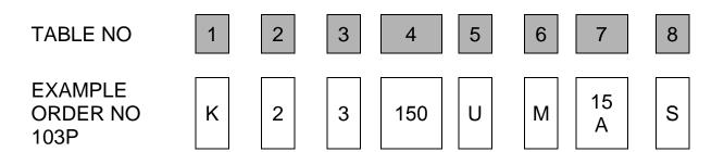
**Example Order No. =** Type 103P T/C-K ; 1/8" sheath diameter ; Inconel 600 sheath material ; 150mm long ; ungrounded measuring junction ; 1/2 N.P.T process connection ; cast aluminum head ; standard calibration.
