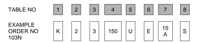
**Example Order No. =** Type 103N T/C-K ; 1/8" sheath diameter ; Inconel 600 sheath material ; 150mm long ; ungrounded measuring junction ; 1/2 N.P.T connection ; aluminum connection head ; standard accuracy.
