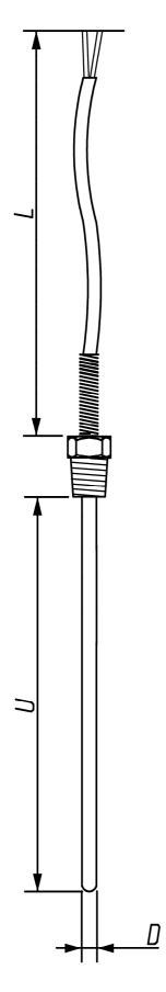
101 is a standard sensor suitable for use with basic applications where there is no need of connection head or not for such enough space connection head.
