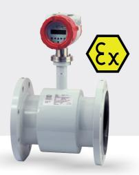
An electrically conductive medium flowing through an orientated magnetic field, in accordance to Faraday's law of induction, will induce a voltage proportional to the mean flow velocity rate and hence the volumetric flow.
